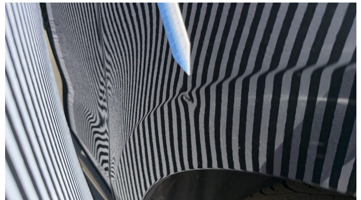
Damage 4: Mudguard - right side: Mudguard - right side - Dent / paintcoat damage - Repair and paint
