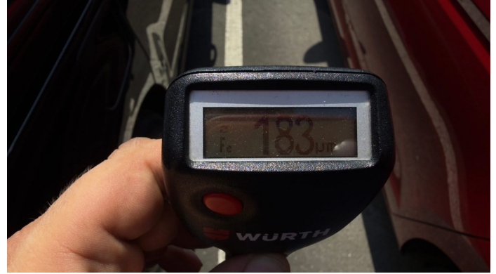
Repainting 1: Boot lid / rear door, Side panel - rear right side, Door - rear right side
