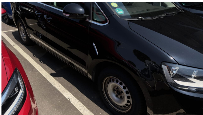
Damage 4: Mudguard - right side: Mudguard - right side - Dent / paintcoat damage - Repair and paint
