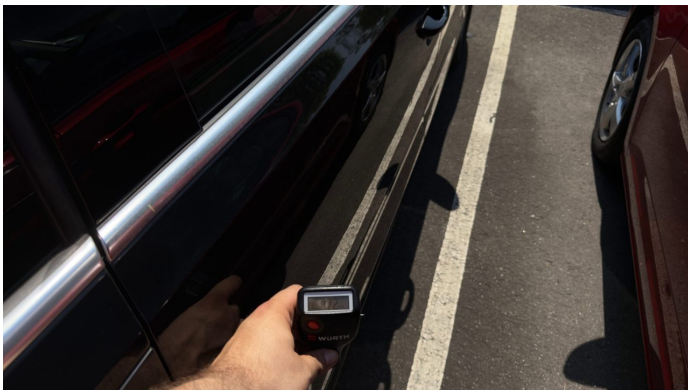
Repainting 1: Boot lid / rear door, Side panel - rear right side, Door - rear right side
