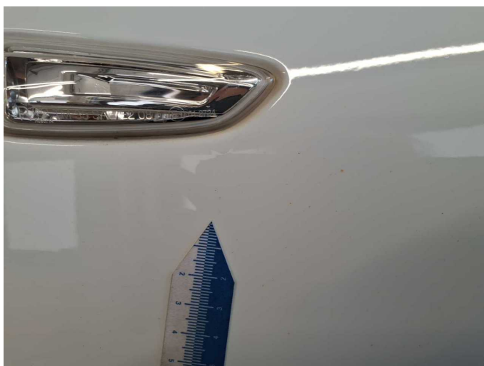
Damage 2: Mudguard - right side: Mudguard - right side (Lackläufer) - Paint defect - Cover / polish
