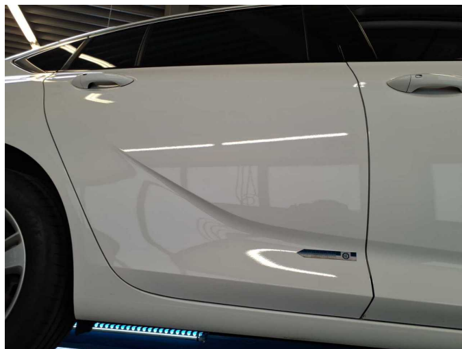
Damage 4: Door - rear right side: Door (Lack Pickel) - Paint defect - Smart repair
