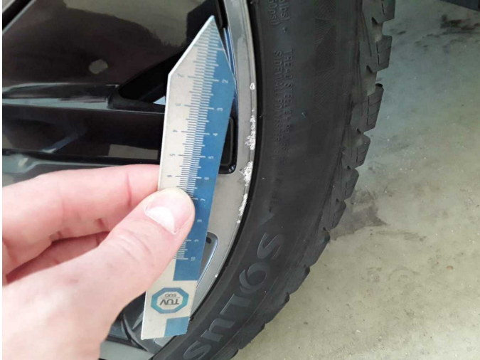
Damage 5: Wheel / tyres: Alloy rim - rear right side - Scratch(es) - Replace
