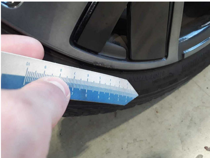
Damage 3: Wheel / tyres: Alloy rim - front left side - Scratch(es) - Loss in value
