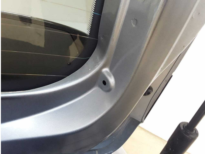
Damage 2: Trim / covers: Boot lid - interior trim (Aufhänger fehlt) - Differs from the original configuration - Replace
