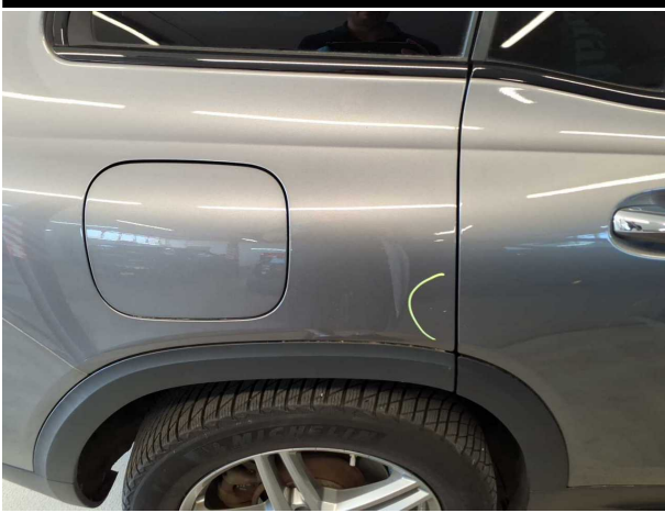
Damage #6: Side panel - rear right side: Side panel - Scratched - Smart repair
