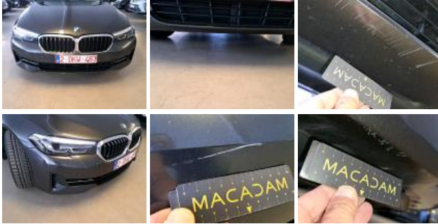
Bumper grille, Broken, Replace
