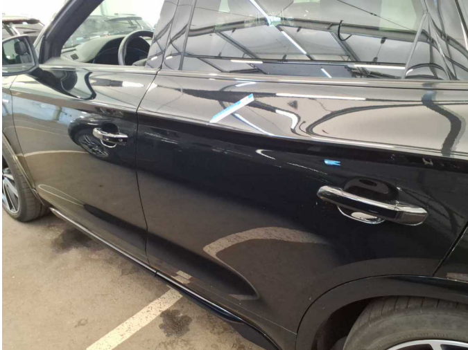
Damage 1: Door - rear left side: Door - Scratched - Smart repair
