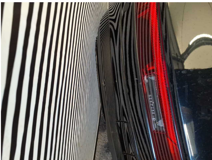
Damage 2: Rear bumper: Spoiler (& Lackschaden) - Deformed - Replace
