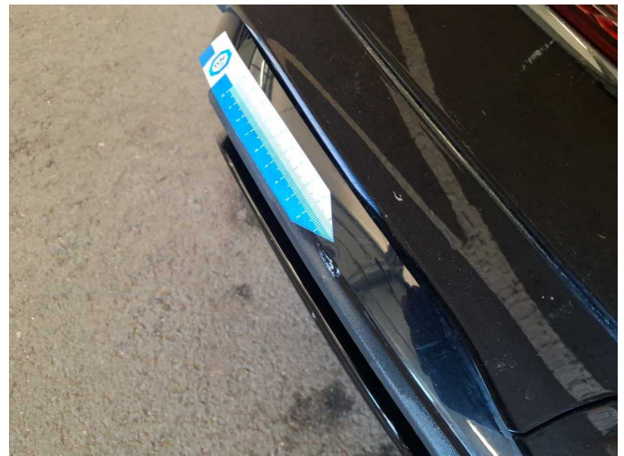
Damage 2: Rear bumper: Spoiler (& Lackschaden) - Deformed - Replace
