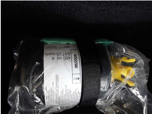
Damage #1: Equipment: Tirefit filler - Expired - Replace
