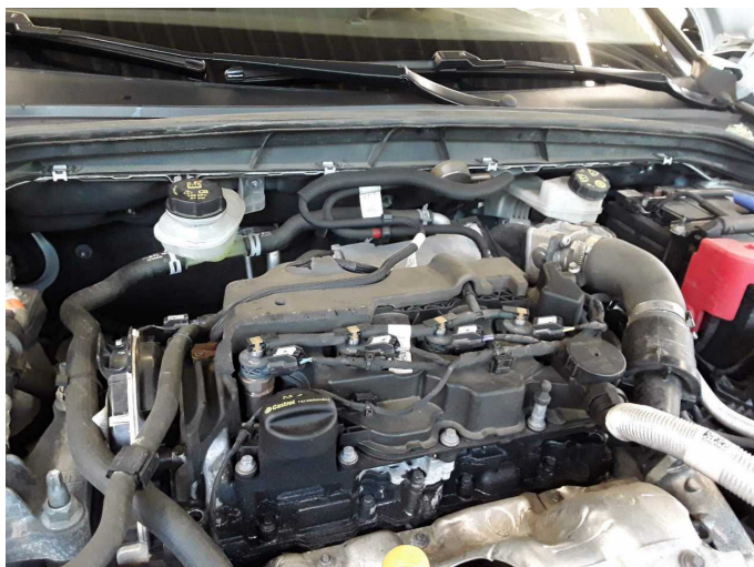
Damage 1: Engine: Engine cover - Damaged - Replace
