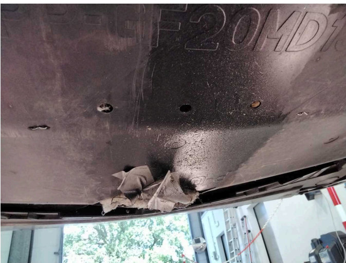
Damage 9: Body: Underbody paneling (Ölfeucht) - Perform diagnosis
