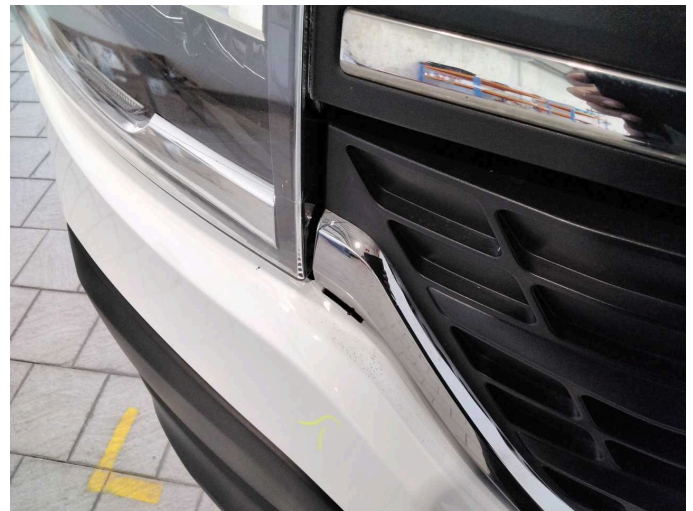
Damage 3: Front bumper: Grille - Malposition - Perform diagnosis
