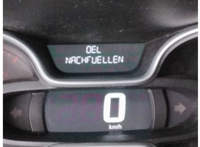
Damage 2: Instrument panel: Indicator light (Öl nachfüllen) - on - Perform diagnosis
