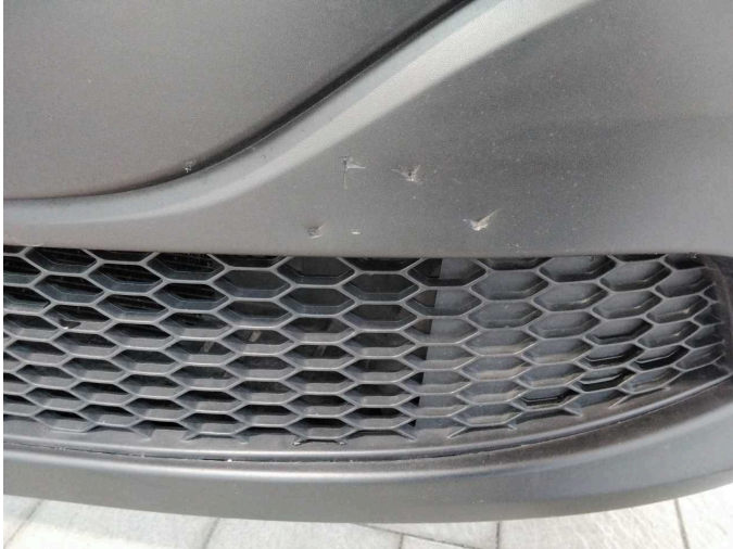
Damage 10: Front bumper: Front bumper - Damaged - Loss in value
