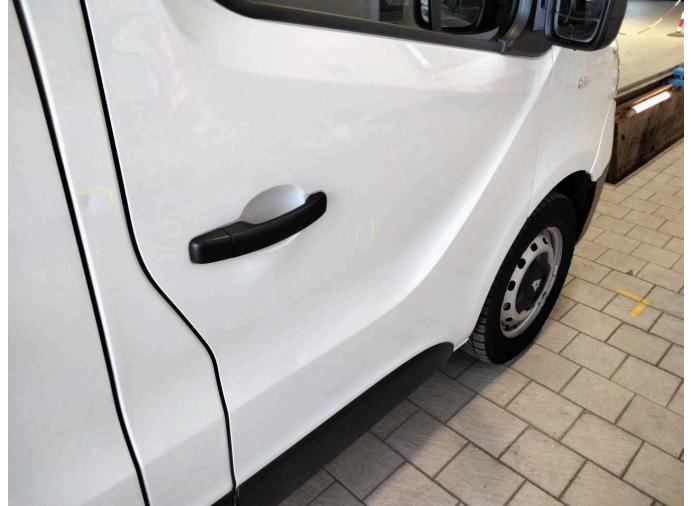
Damage 11: Door - front right side: Door - Dent / paintcoat damage - Smart repair
