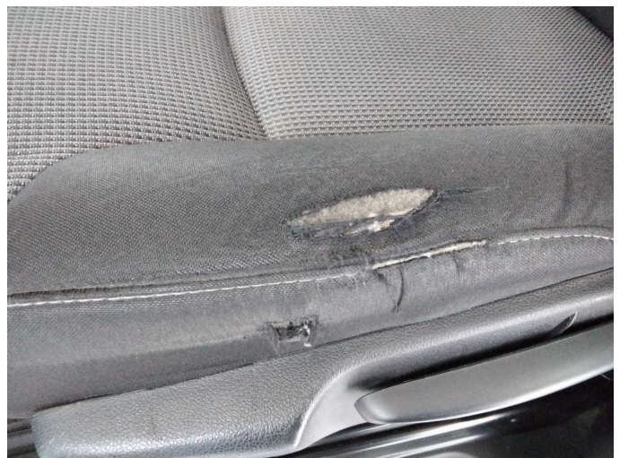
Damage 12: Seat - front: Seat cover - left side - Broken / torn - Replace
