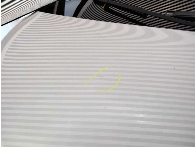
Wear and tear 7: Bonnet: Bonnet - dent(s) - Smooth repair work
