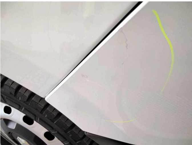
Damage 8: Front bumper: Front bumper (Rechte Seite) - Paint defect - Smart repair
