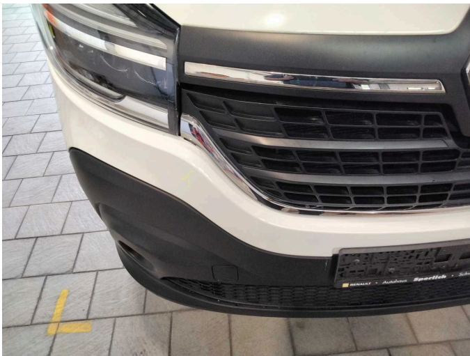
Damage 3: Front bumper: Grille - Malposition - Perform diagnosis
