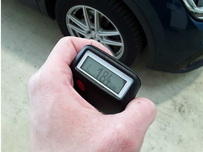
Repainting 1: Mudguard - right side, Side panel - rear right side
