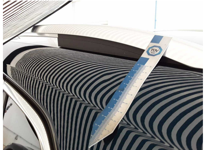
Damage 3: Roof: Roof rail - left side - dent(s) - Smart repair
