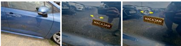
Sill trim R, Scratch(es), Paint
