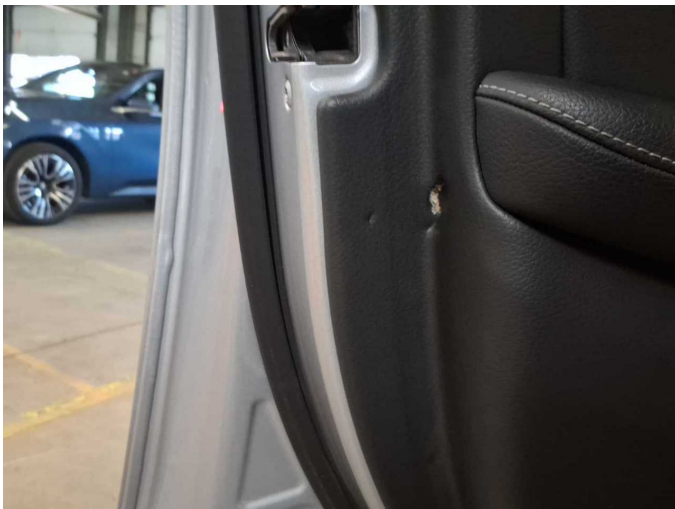
Damage 10: Trim / covers: Door trim - front left side - Broken / torn - Loss in value
