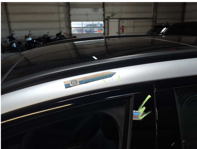
Damage 11: Roof: Roof rail - left side - Dent / paintcoat damage - Repair and paint
