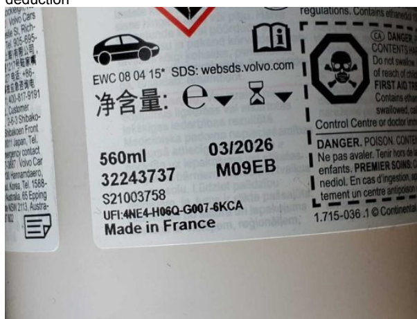
Damage #4: Equipment: Tirefit filler - Expired - Replace
