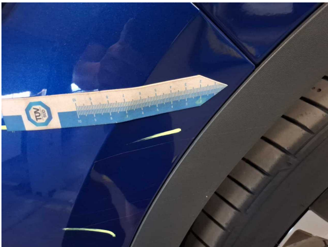
Damage 6: Front bumper: Front bumper - Scratched - Paint
