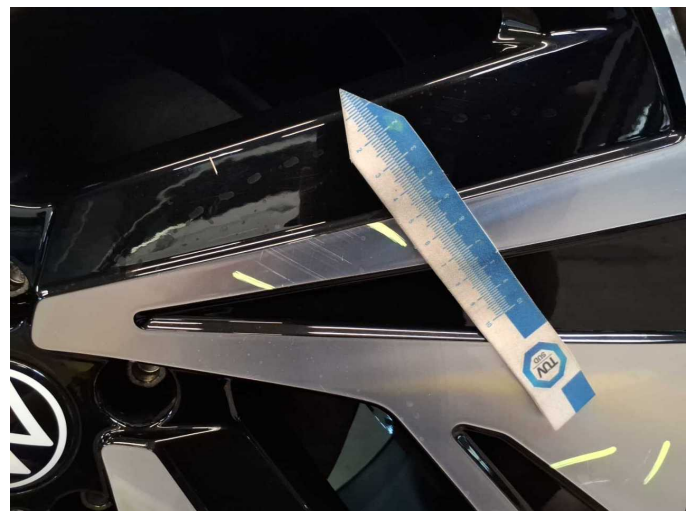
Damage 1: Wheel / tyres: Alloy rim - rear left side - Scratch(es) - Loss in value
