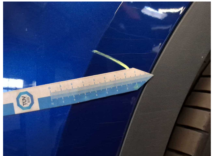
Damage 6: Front bumper: Front bumper - Scratched - Paint
