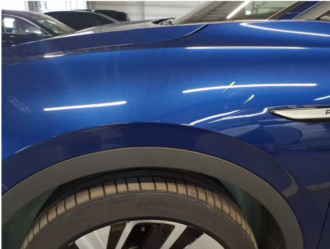
Damage 5: Mudguard - left side: Mudguard - left side - Scratched - Smart repair
