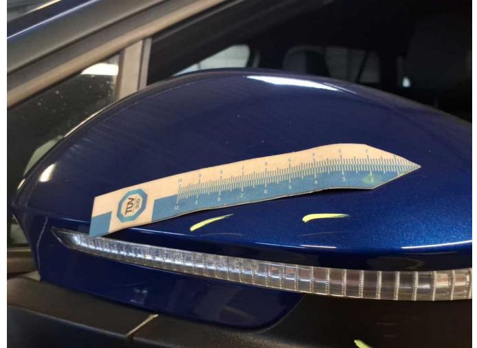
Damage 2: Wing mirror - left side: Cap - Scratch(es) - Smart repair
