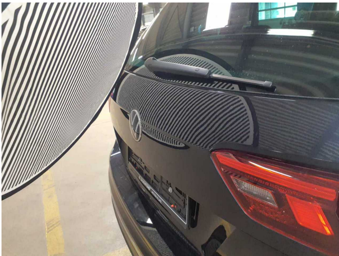
Damage 4: Boot lid / rear door: Boot lid - Deformed - Paint
