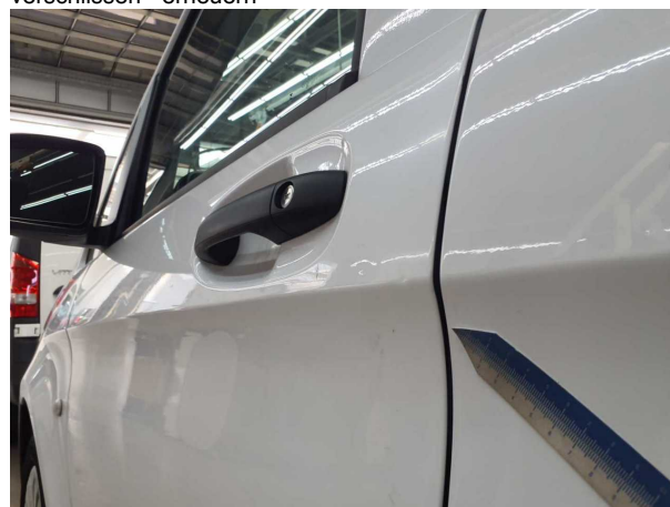
Beschädigung #12: Tür vorn links: Tür - Delle / Lackschaden - Smart Repair
