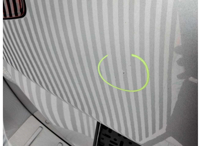
Damage 4: Boot lid / rear door: Boot lid - Dent / paintcoat damage - Repair and paint
