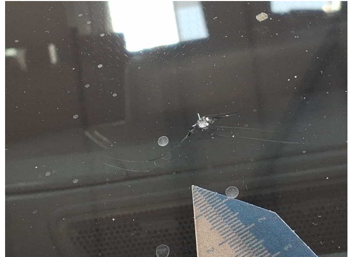
Damage 4: Vehicle glazing: Windscreen - Broken / torn - Replace
