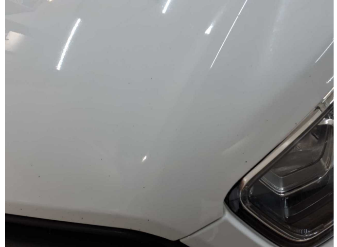
Damage 3: Bonnet: Bonnet - Stone chips - Paint
