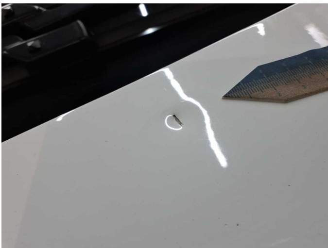
Damage 3: Bonnet: Bonnet - Stone chips - Paint
