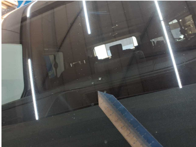
Damage 4: Vehicle glazing: Windscreen - Broken / torn - Replace
