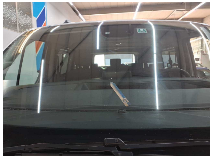
Damage 4: Vehicle glazing: Windscreen - Broken / torn - Replace
