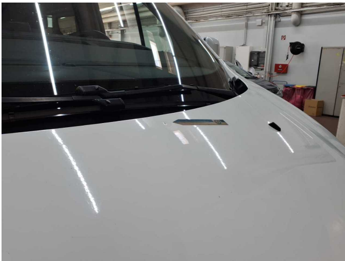
Damage 3: Bonnet: Bonnet - Stone chips - Paint
