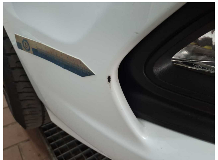
Damage 1: Front bumper: Spoiler - Scratch(es) - Smart repair
