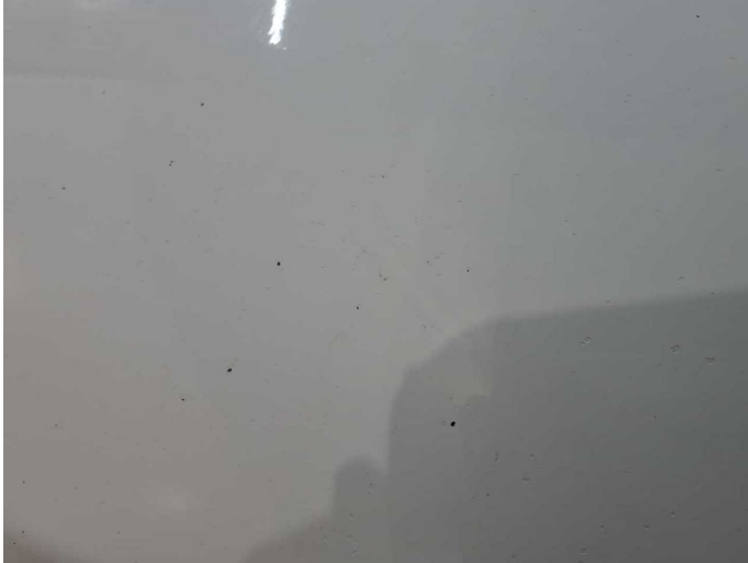
Damage 3: Bonnet: Bonnet - Stone chips - Paint
