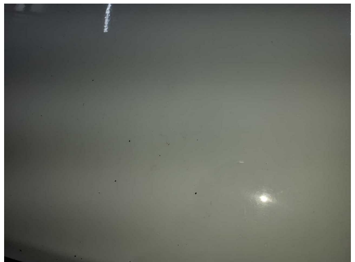
Damage 3: Bonnet: Bonnet - Stone chips - Paint
