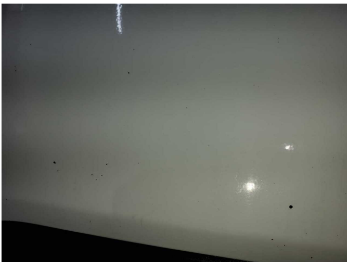
Damage 3: Bonnet: Bonnet - Stone chips - Paint
