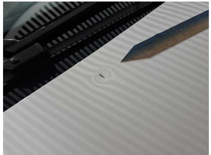
Damage 3: Bonnet: Bonnet - Stone chips - Paint
