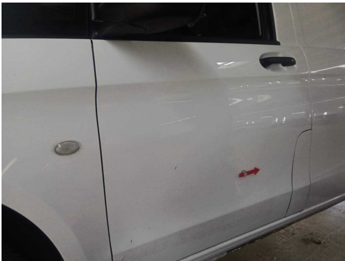
Damage 5: Door - front left side: Door - Dent / paintcoat damage - Repair and paint
