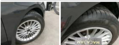
Wheel cover FR, Missing, Replace
