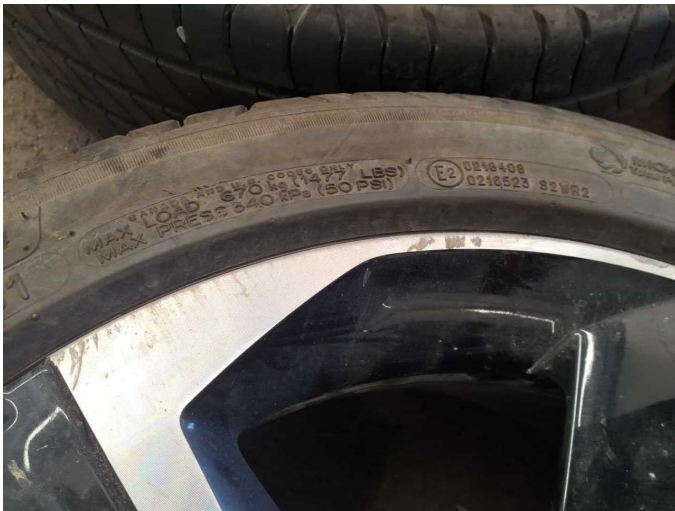
Damage 4: 2nd wheel set: 1 alloy rim - Scratched - Replace
