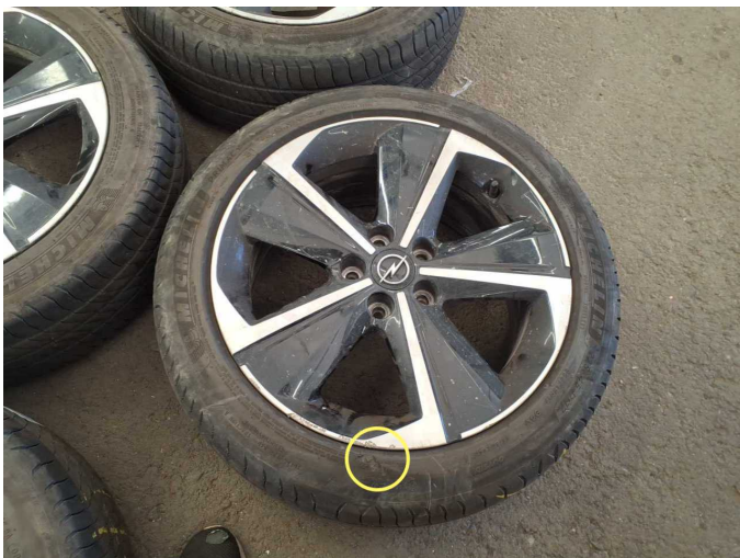
Damage 2: 2nd wheel set: 1 tyre - Damaged - Replace
