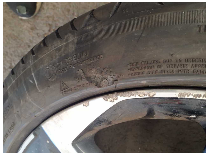
Damage 2: 2nd wheel set: 1 tyre - Damaged - Replace
