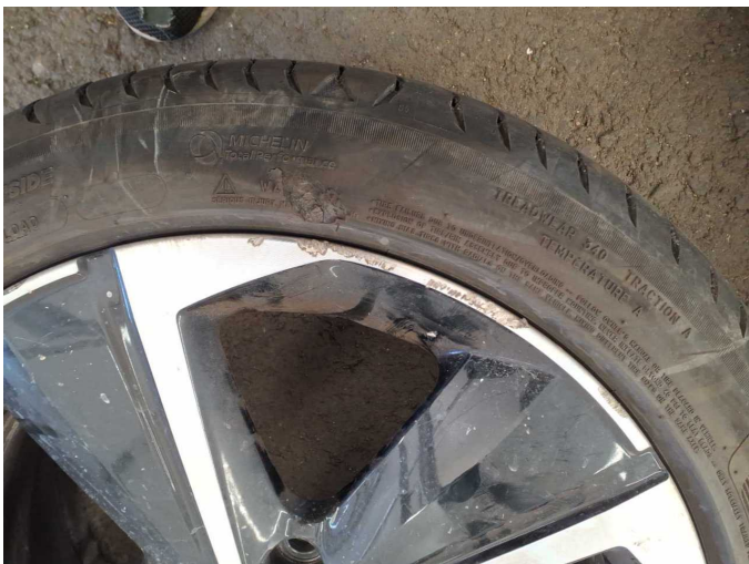
Damage 5: 2nd wheel set: 1 alloy rim - Scratched - Replace
