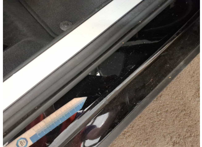
Damage 1: Sill - right side: Sill - Dent / paintcoat damage - Smart repair
