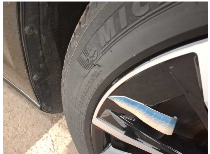
Damage 2: Wheel / tyres: Tyre - front right side (nicht fahrbereit) - Broken / torn - Replace
