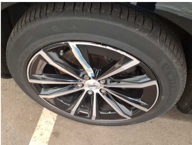
Damage 5: Wheel / tyres: Alloy rim - rear right side - Scratched - Loss in value
