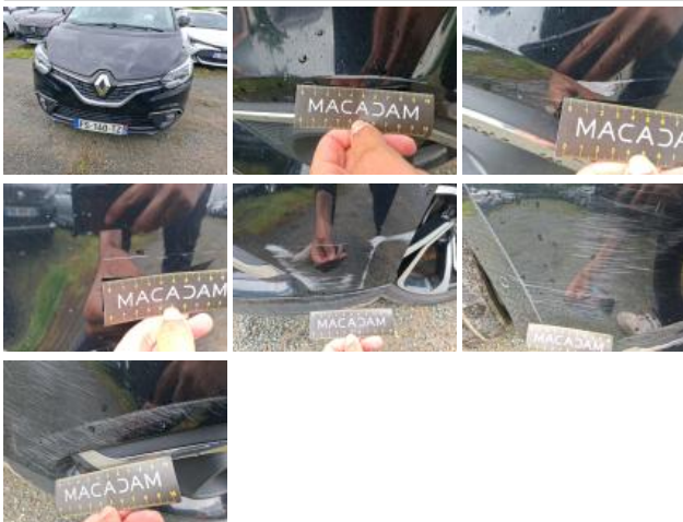
Door RR, Dent(s), Repair and paint (complete)
