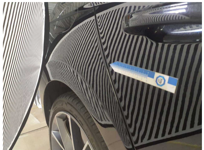
Damage 2: Side panel - rear right side: Side panel (Welliger Untergrund) - Unprofessionally repaired - Repair and paint
