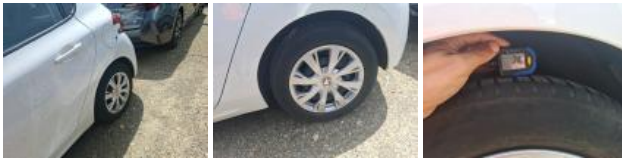
Tyre RR, Out of tolerance, Replace
