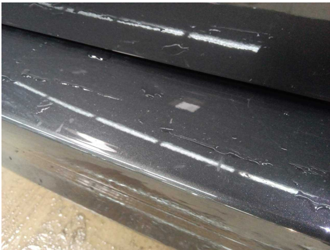
Damage 4: Rear bumper: Rear bumper - Scratch(es) - Paint
