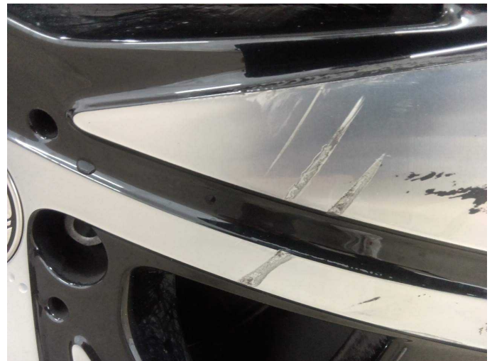
Damage 3: Wheel / tyres: Alloy rim - front right side - Scratch(es) - Replace
