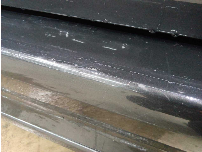
Damage 4: Rear bumper: Rear bumper - Scratch(es) - Paint
