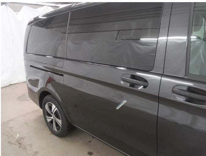
Damage 5: Sliding door, right: Sliding door - Dent / paintcoat damage - Repair and paint
