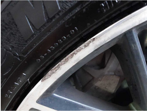
Wear and tear 2: Wheel / tyres: Alloy rim - front right side (Materialabtrag) - Scratched - No deduction
