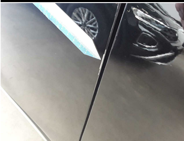
Damage #3: Door - front right side: Door edge - Scratched - Smart repair
