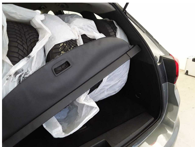
Damage 9: Interior: Boot cover / roller cover - Broken / torn - Replace
