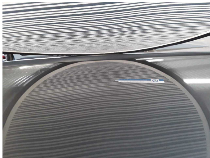
Damage 1: Roof: Roof - dent(s) - Smooth repair work
