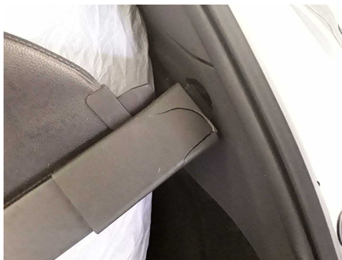
Damage 9: Interior: Boot cover / roller cover - Broken / torn - Replace
