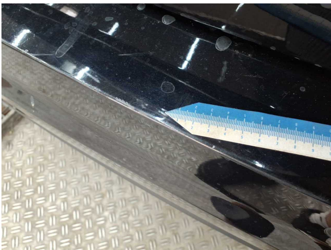
Damage 4: Rear bumper: Rear bumper - Scratch(es) - Paint
