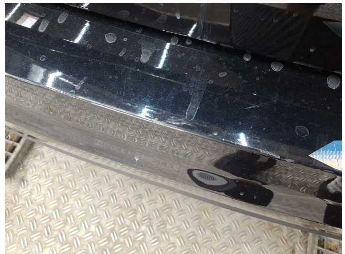
Damage 4: Rear bumper: Rear bumper - Scratch(es) - Paint
