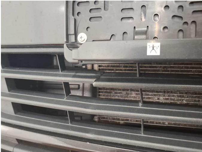
Damage 3: Front bumper: Air-inlet grille - Broken / torn - Replace
