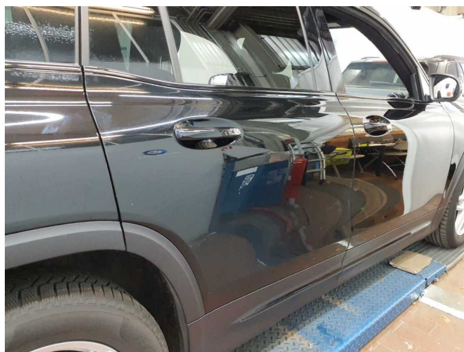
Damage 11: Door - rear right side: Door (Orangenhaut) - Unprofessionally repaired - Paint
