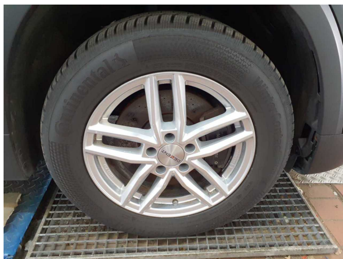
Damage 10: Braking system: Brake discs and brake pads - front - Corrosion - Replace
