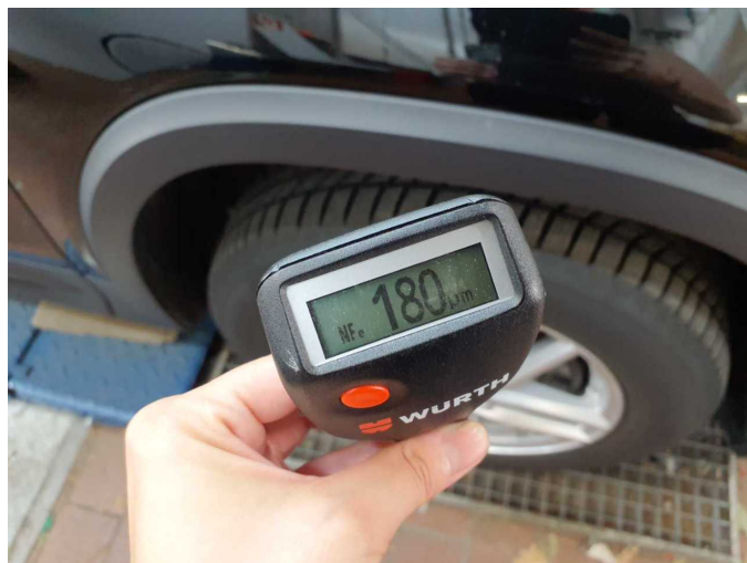
Repainting 1: Mudguard - left side, Mudguard - right side
