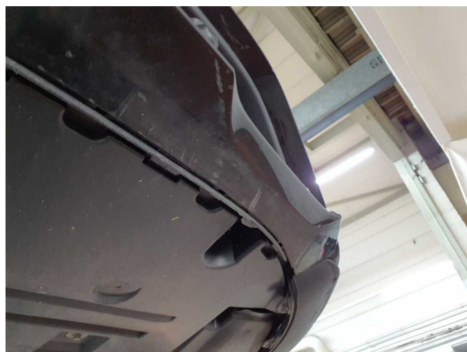
Damage 6: Front bumper: Spoiler - Scratch(es) - Paint
