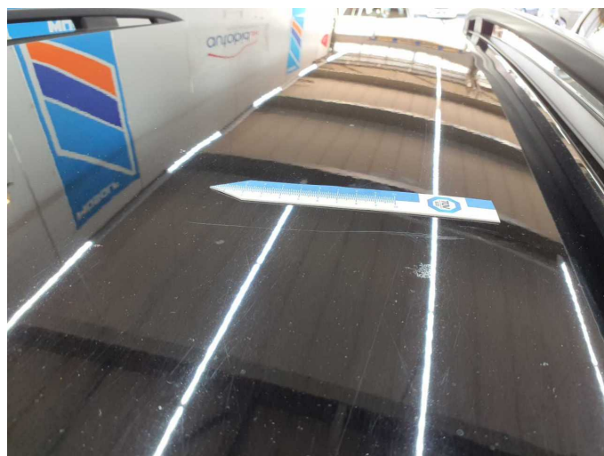
Damage 13: Roof: Roof - Scratch(es) - Paint
