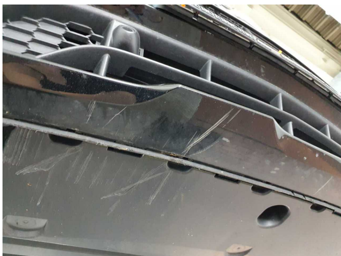
Damage 6: Front bumper: Spoiler - Scratch(es) - Paint
