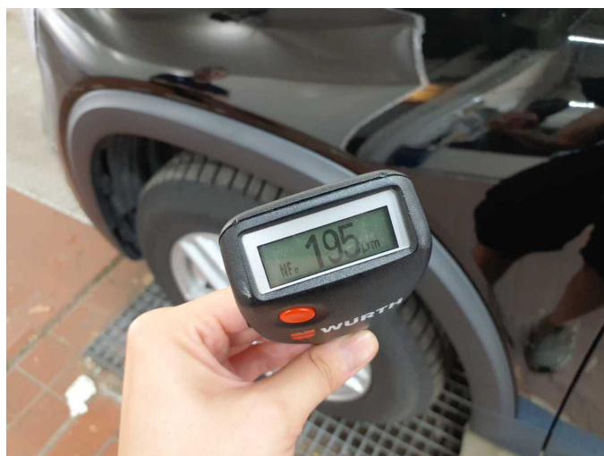
Repainting 1: Mudguard - left side, Mudguard - right side
