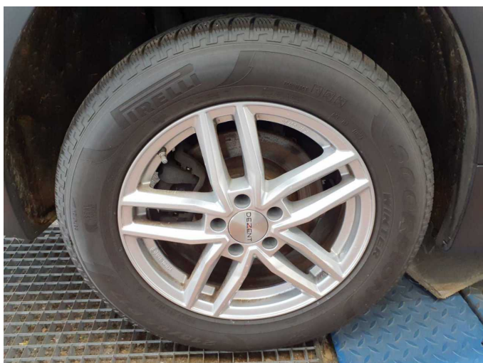
Damage 9: Braking system: Brake discs and pads - rear - Corrosion - Replace
