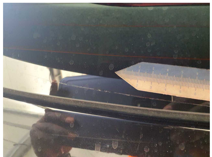
Damage 11: Vehicle glazing: Rear window - Scratch(es) - Replace
