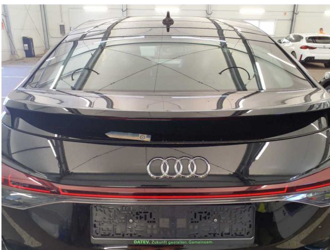
Damage 11: Vehicle glazing: Rear window - Scratch(es) - Replace
