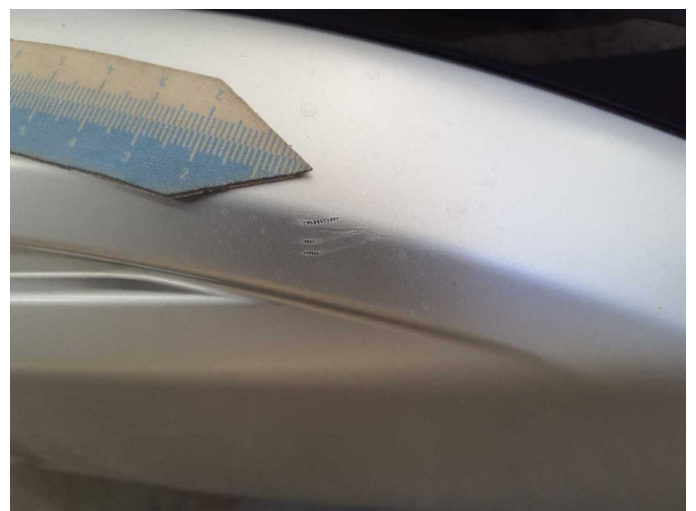
Damage 8: Rear bumper: Spoiler - Scratched - Replace
