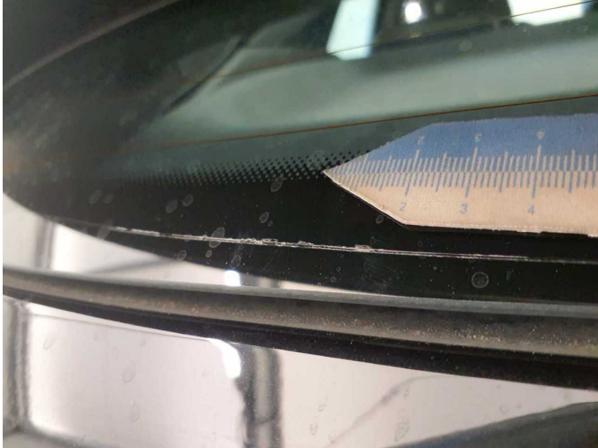
Damage 11: Vehicle glazing: Rear window - Scratch(es) - Replace
