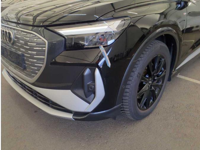
Damage 10: Front bumper: Front bumper - Scratched - Paint
