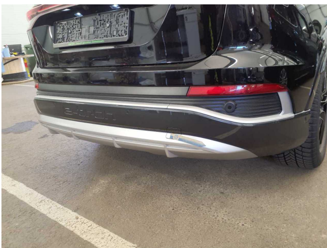
Damage 8: Rear bumper: Spoiler - Scratched - Replace
