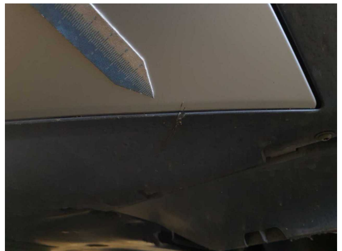
Damage 7: Front bumper: Spoiler (Unterhalb) - Scratch(es) - Loss in value
