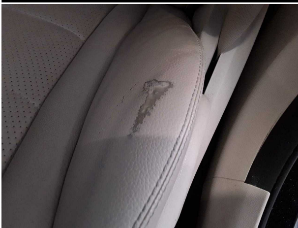
Damage #5: Seat - front: Seat cover - left side - Porous / cracked - Replace
