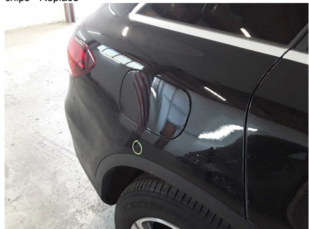
Damage #8: Side panel - rear right side: Side panel - dent(s) - Repair and paint
