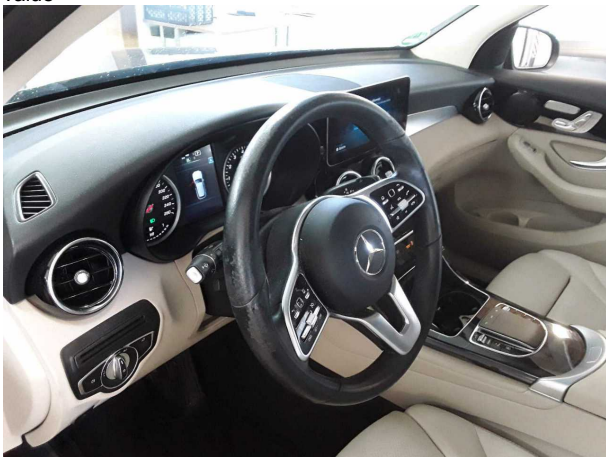
Damage #4: Steering system: Steering wheel (starker) - Abrasion - Loss in value
