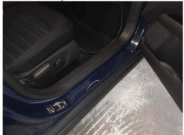
Damage #3: Sill - right side: Sill - Scratched - Smart repair
