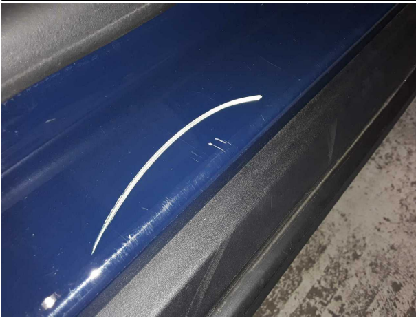
Damage #3: Sill - right side: Sill - Scratched - Smart repair
