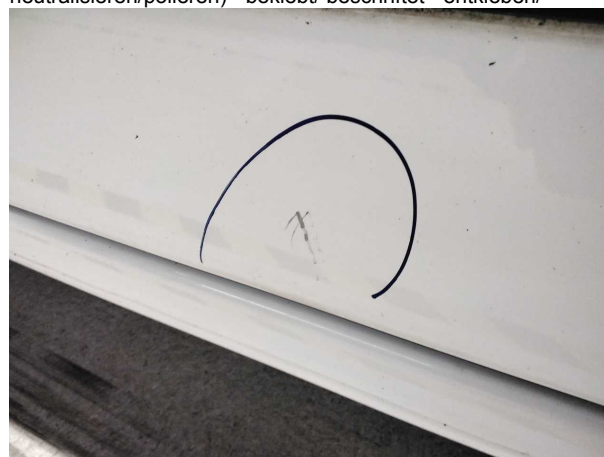
Beschädigung #9: Tür vorn links: Tür - Kratzer - Smart Repair
