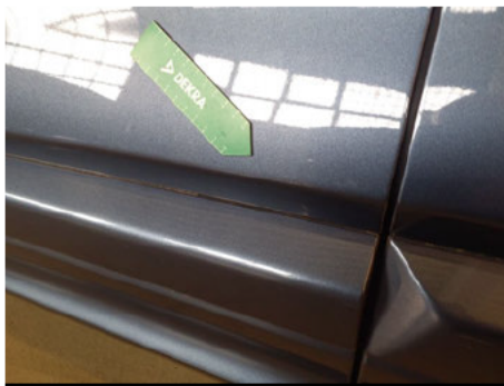
Tür / Vorne Links / Kratzer
