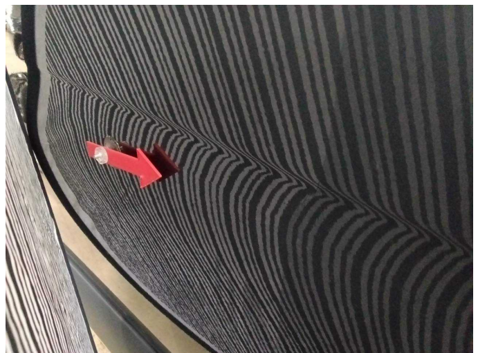
Damage 2: Sliding door, right: Sliding door - dent(s) - Smooth repair work
