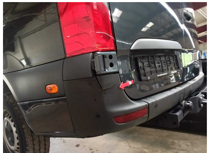
Damage 5: Rear bumper: Bumper - rear left side (Eckteil) - Broken / torn - Replace
