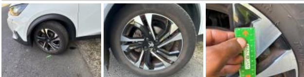
Wing trim FL, Scratch(es), Replace
