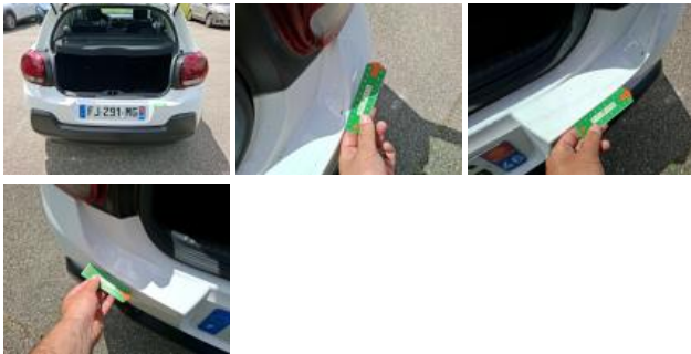
Boot lid covering R, Scratch(es), Replace
