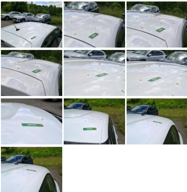
Roof, Hail damage, Repair and paint (complete)
