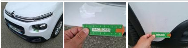
Bumper moulding F, Scratch(es), Replace
