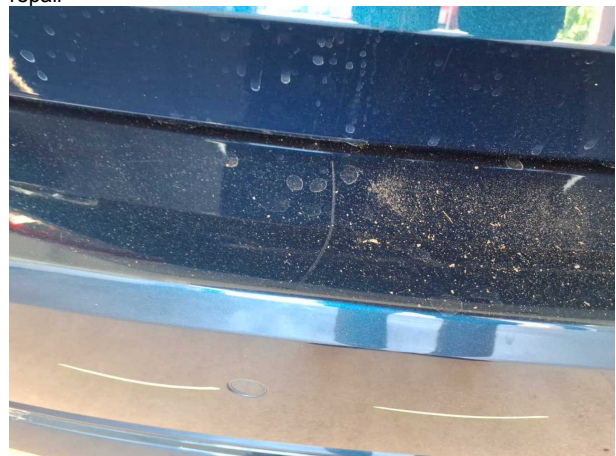
Damage #4: Rear bumper: Rear bumper - Scratched - Smart repair
