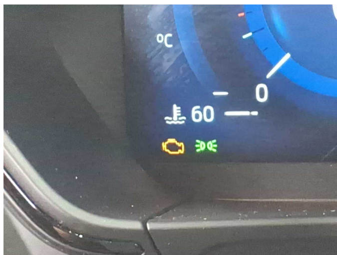
Damage 6: Instrument panel: Indicator light (Motorkontrolleuchte) - on - Perform diagnosis
