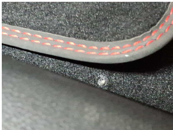
Damage 3: Trim / covers: Carpet - Burn hole (cigarettes) - Smart repair
