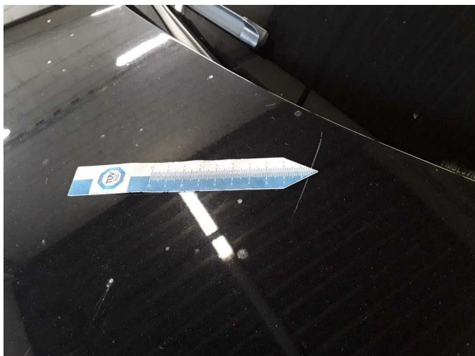
Damage 4: Bonnet: Bonnet - Scratch(es) - Paint
