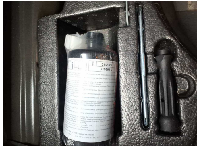
Damage 1: Equipment: Tirefit filler - Expired - Replace
