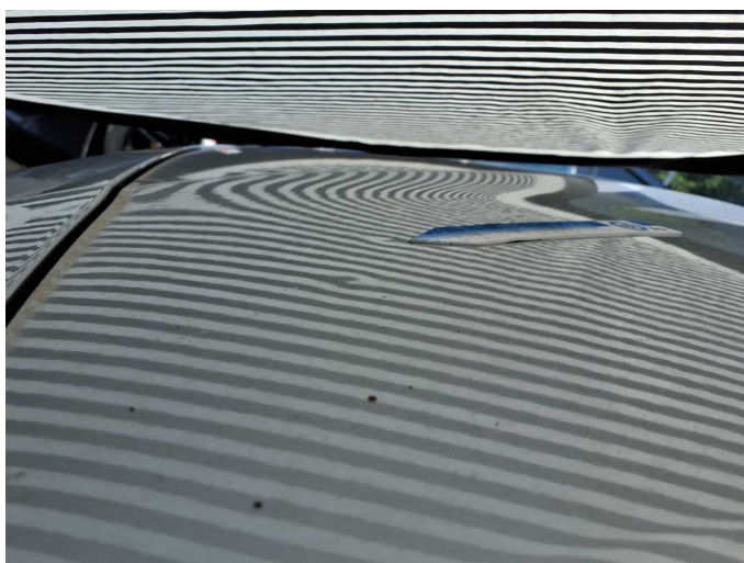
Damage 4: Bonnet: Bonnet - dent(s) - Smooth repair work
