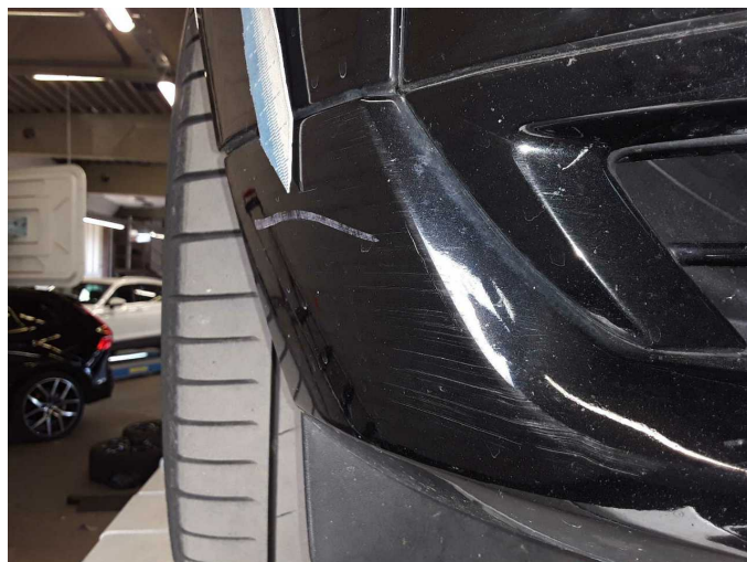
Damage 11: Front bumper: Front bumper - Scratch(es) - Paint
