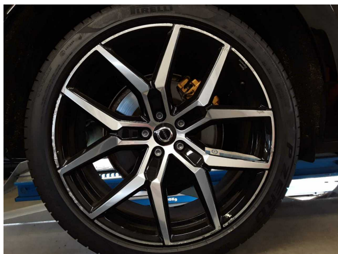
Damage 12: Wheel / tyres: Alloy rim - rear right side (Materialabtrag) - Scratched - repair according to calculation
