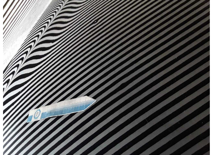
Damage 5: Bonnet: Bonnet (5 Dellen) - dent(s) - Smooth repair work
