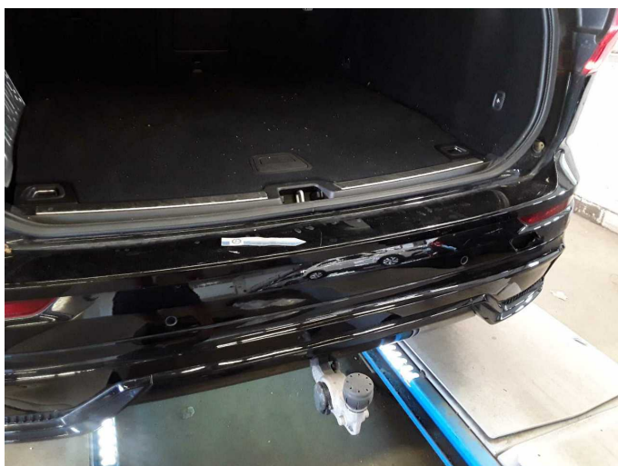
Damage 10: Rear bumper: Rear bumper - Scratch(es) - Paint
