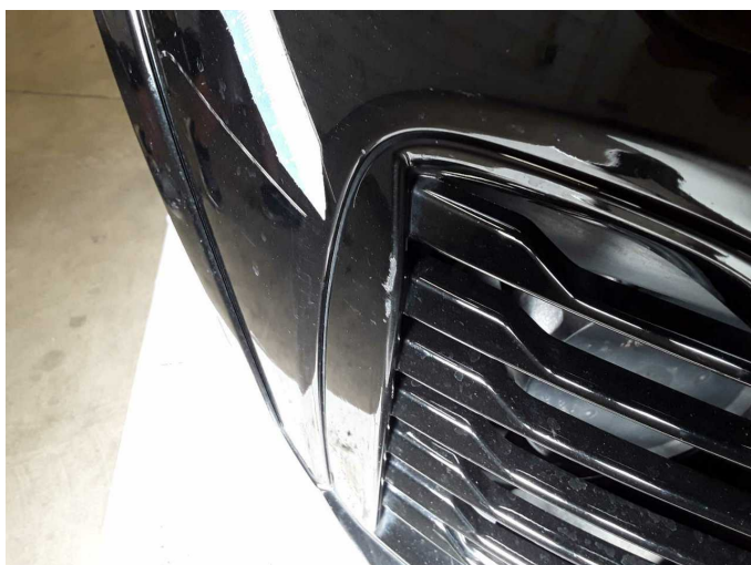
Damage 11: Front bumper: Front bumper - Scratch(es) - Paint
