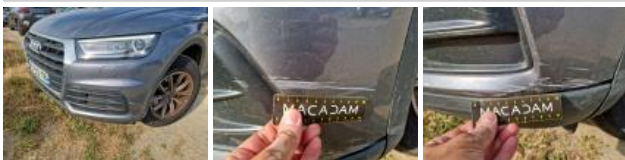
Bumper moulding FL, Scratch(es), Replace
