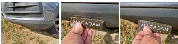
Bumper moulding FL, Scratch(es), Replace
