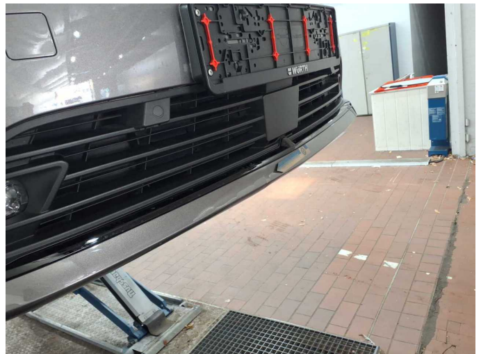
Damage 7: Front bumper: Front bumper - Deformed - Replace
