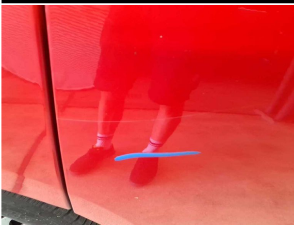
Damage #14: Sliding door, right: Sliding door with glass panel - Dent / paintcoat damage - Repair and paint
