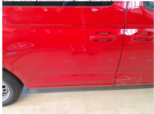
Damage #14: Sliding door, right: Sliding door with glass panel - Dent / paintcoat damage - Repair and paint
