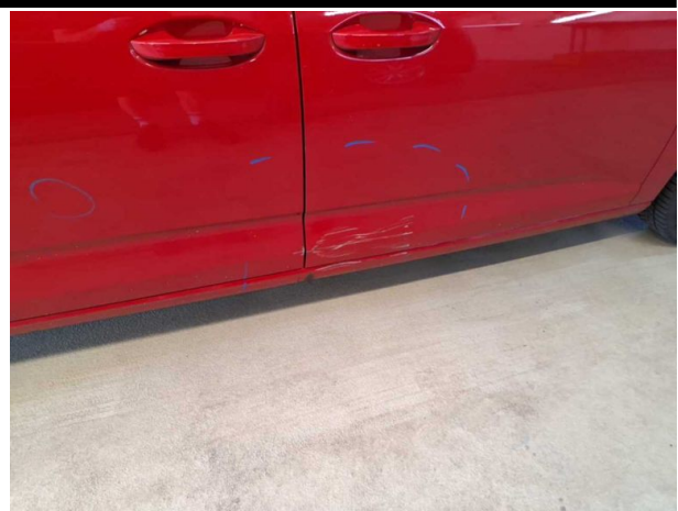
Damage #11: Sill - right side: Sill - Deformed - Repair and paint
