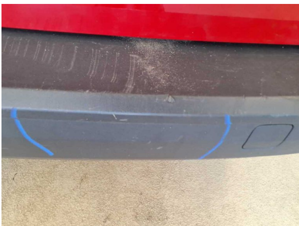
Damage #10: Rear bumper: Rear bumper (unpainted) - Scratched - Loss in value
