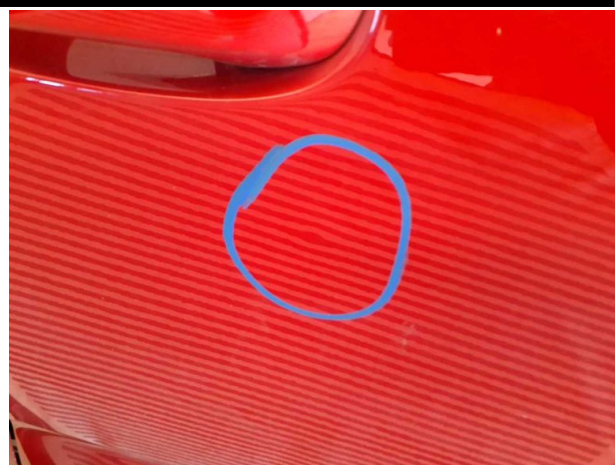
Damage #13: Sliding door - left side: Sliding door with glass panel - Dent / paintcoat damage - Repair and paint
