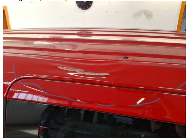
Damage #16: Roof: Roof - Deformed - Repair and paint
