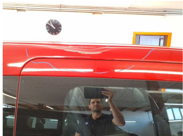
Damage #12: Roof: Roof rail - right side - Dent / paintcoat damage - Repair and paint
