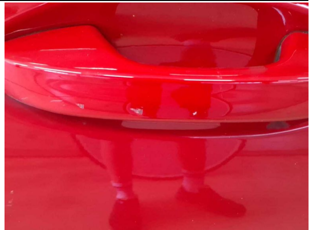
Damage #8: Door - front right side: Door handle - outside - Scratched - Smart repair
