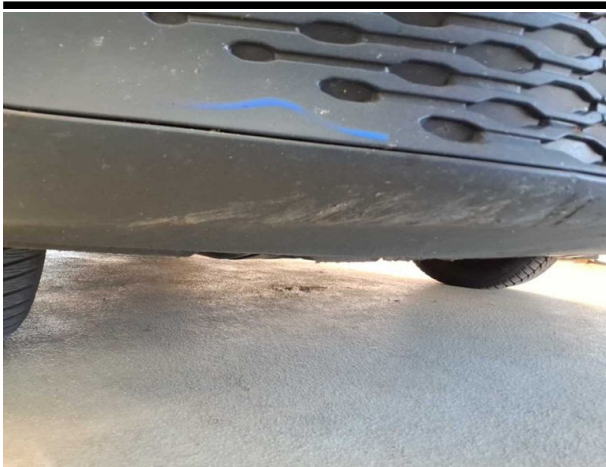
Damage #7: Front bumper: Front bumper (unpainted) - Scratched - Loss in value
