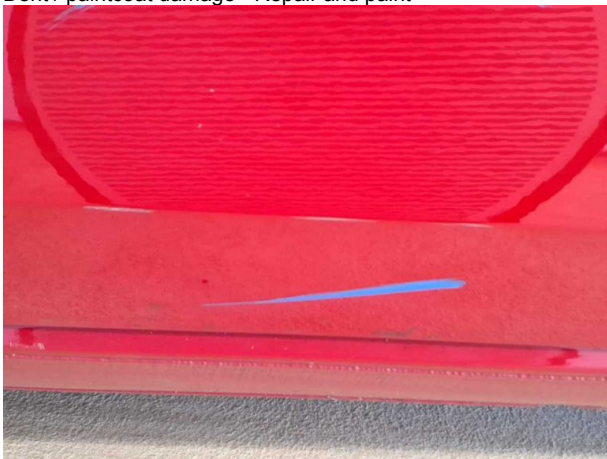
Damage #13: Sliding door - left side: Sliding door with glass pane... Dent / paintcoat damage - Repair and paint
