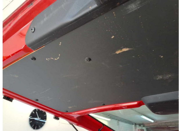
Damage #4: Trim / covers: Boot lining - Scratched - Loss in value
