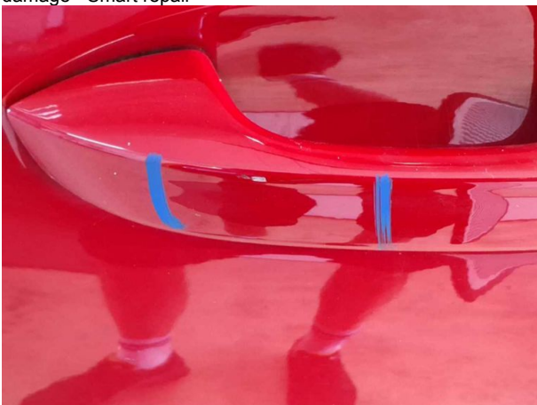
Damage #6: Door - front left side: Door handle - outside - Scratched - Smart repair
