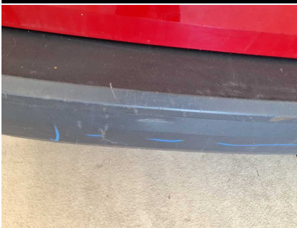
Damage #10: Rear bumper: Rear bumper (unpainted) - Scratches... Loss in value
