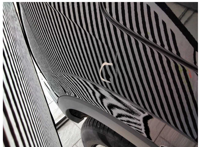
Wear and tear 4: Side panel - rear right side: Side panel - dent(s) - Smooth repair work
