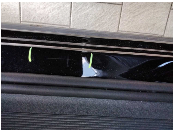
Damage 2: Body: C-pillar - left side - Dent / paintcoat damage - Smart repair
