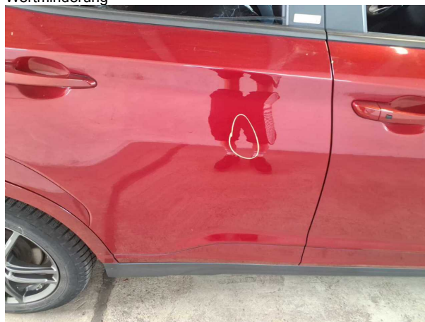
Beschädigung #4: Tür hinten rechts: Tür - Delle / Lackschaden - Smart Repair
