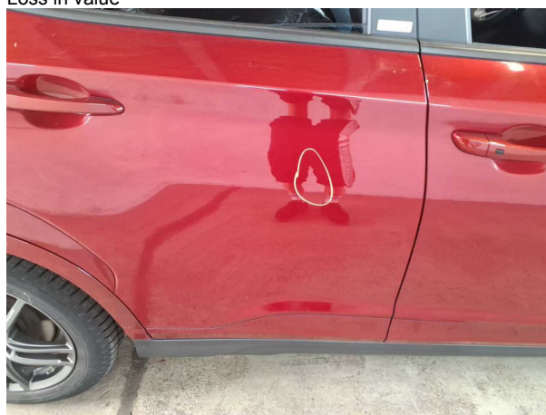
Damage #4: Door - rear right side: Door - Dent / paintcoat damage - Smart repair
